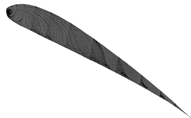
Fig. 10 Surface particle traces on the flap end. \delta_f = 30 deg, \alpha = 10 deg.
